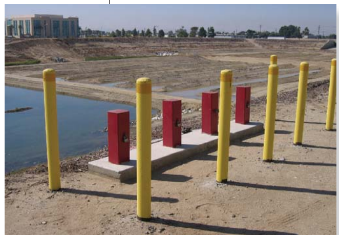
Lysimeters used to monitor compliance
