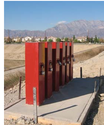
Lysimeters at recharge basin
