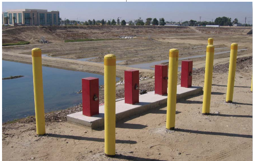
Lysimeters at recharge basin
